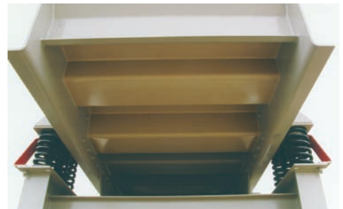
Rigid Box Beam Construction
