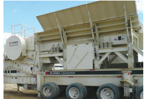
High Capacity Vibrating Grizzly Feeder
